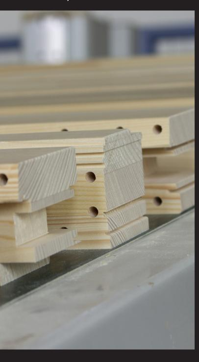
Our doors and windows made of wood or wood-aluminium are produced using laminated, warping-free, solid wood in our plant in Sopron by using the latest manufacturing technologies and by taking into account market needs all the time. We pay great attention on details:
